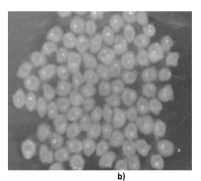
Figure 1: Digital camera Photos of formulation a) Dummy beads without gas forming agent b) Dummy beads with gas forming agent shown centrally air entrapment
